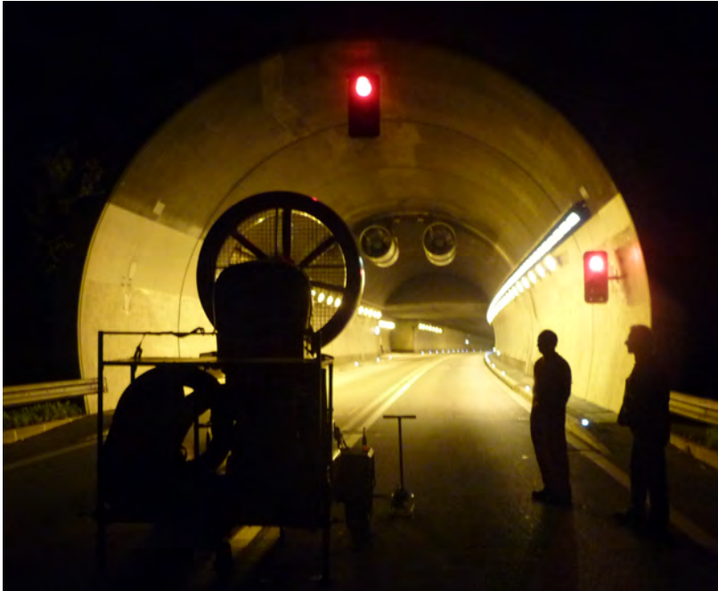
Figure 2. Mobile jet fan for simulations of meteorological pressures
