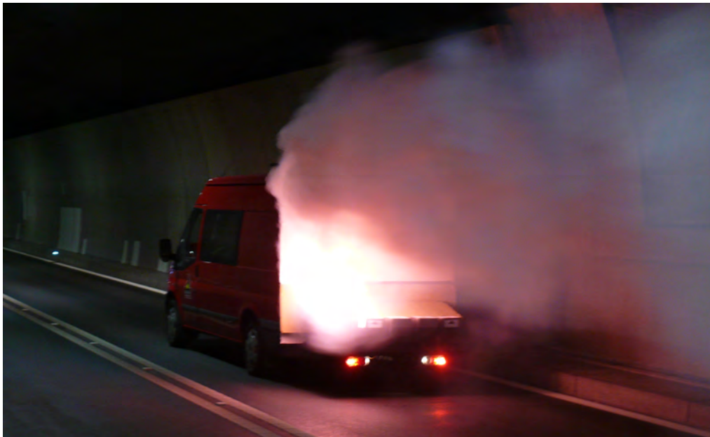
Figure 4. Simulation of a moving burning car
