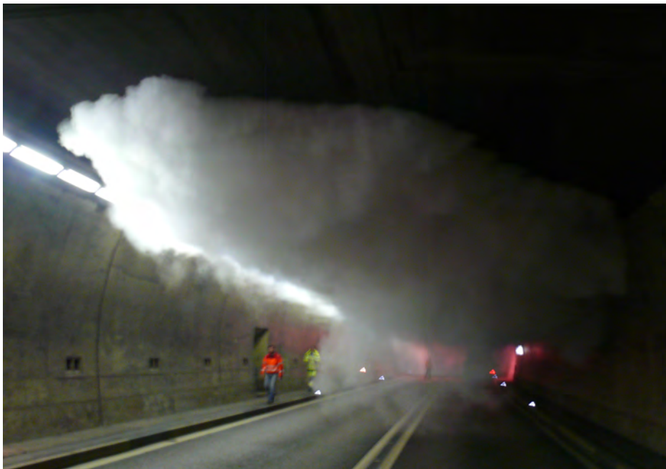
Figure 5. Smoke test in the Isla Bella tunnel
