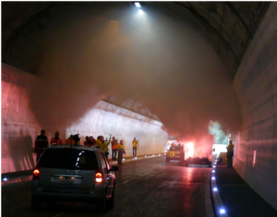
Figure 6. Smoke test in the Saaser tunnel
