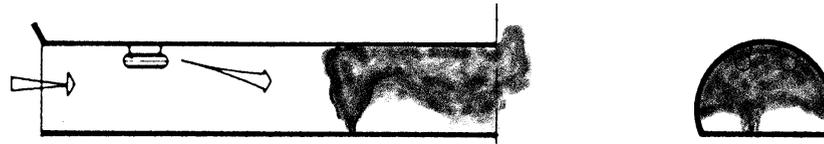
*Fig. 2 Longitudinal ventilation in case of fire*
