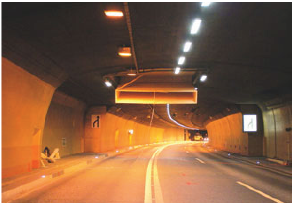
Figure 3.6: Setup of Saccardo nozzle mock-up
