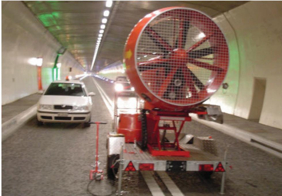
Figure 3.5: Mobile jet fan
